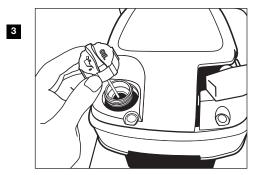
**Step 3** Check oil level. Oil level should always be between the "FULL" and "ADD" marks on the dipstick. Be sure the machine is level when checking the oil level. (Refer to the engine's operating manual for seasonal grades.)
